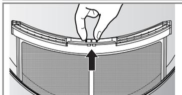
3. Clean the filter by using a vacuum cleaner or rinsing under the tap.
