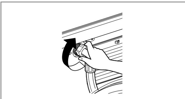
4. Replace the filter and tighten up the inlet hose.
