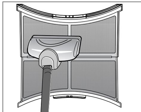
Clean the filter. (Replace the filter if it is damaged.)
