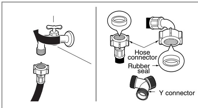
► Step1 : Check rubber seal in the inlet hose.
