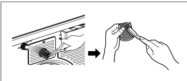
3. Carefully remove the filter from inlet valve and clean the filter using a bristle brush.
