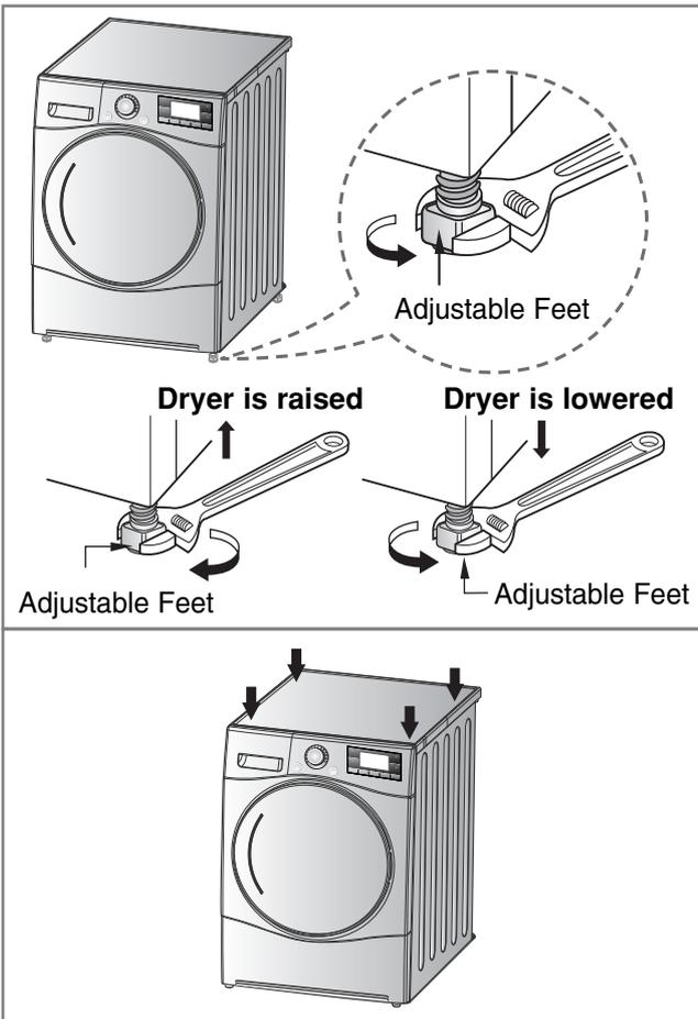
2. If the dryer is not properly level, adjust the front levelling feet as necessary.
