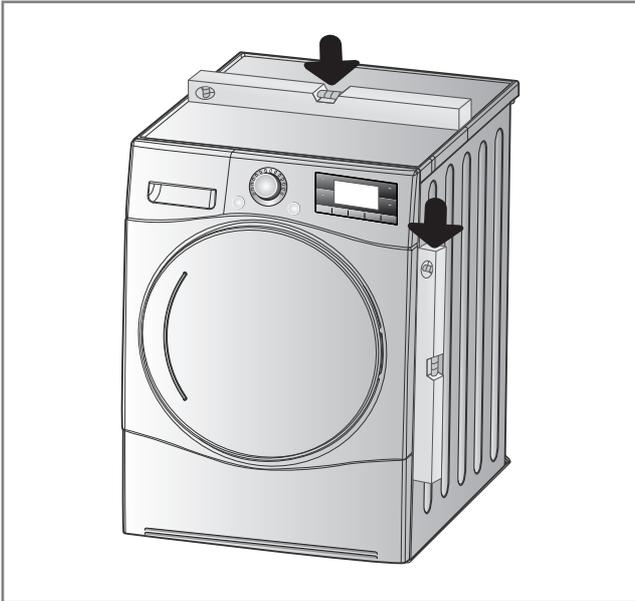
1. Levelling the dryer prevents unnecessary noise and vibration. Place your dryer on a solid, level floor.
